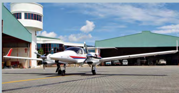
Twin Engine All-Composite Diamond DA-42 Twin Star
