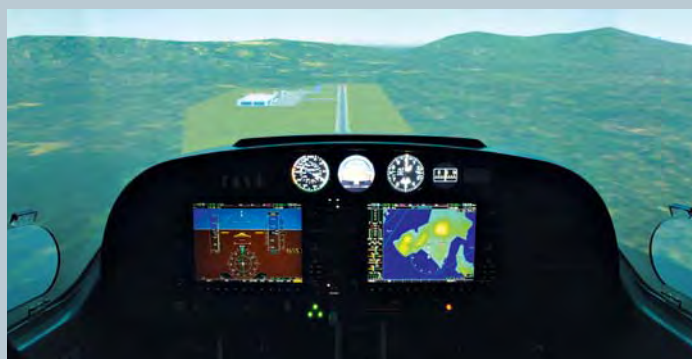
Flight Navigation Procedures Trainer (FNPT) II Simulator ALSIM AL200-DA42
